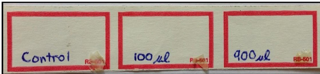
Figure (3-5). Films synthesized with 0.67 wt% alginate, 0.03 mg/ml (0.44 U/ml) enzyme and iron (II). The films are overlaid on top of the words in the bottom right corner. Iron concentrations are 0, 1.67, and 15 mM which correspond to samples labeled: 0, 100 \mu l and 900 \mu l.
